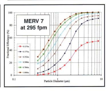
Particle Size Removal Efficiency Conducted by LMS Technologies. (December 2006)
