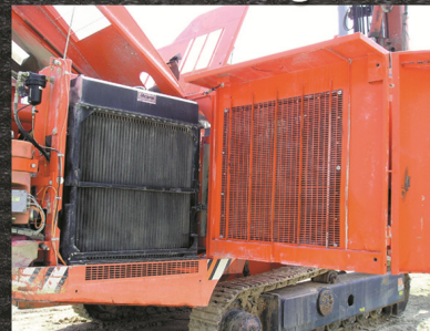
Drilling Rig Air Intake
